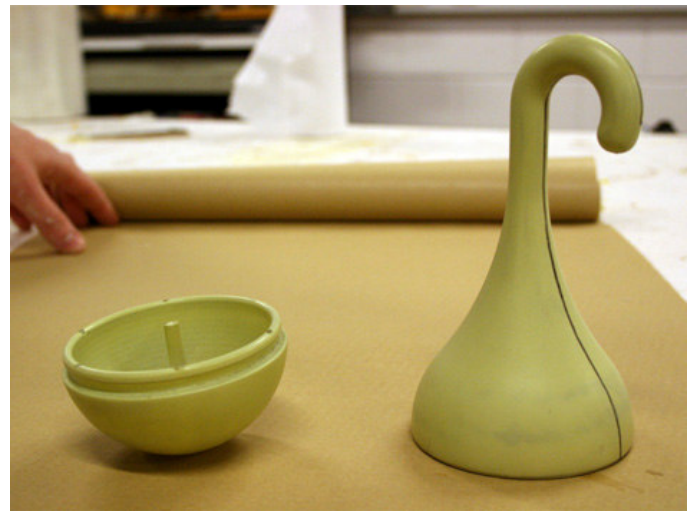
Figure 3.b. Rapid prototyping model used as master model
