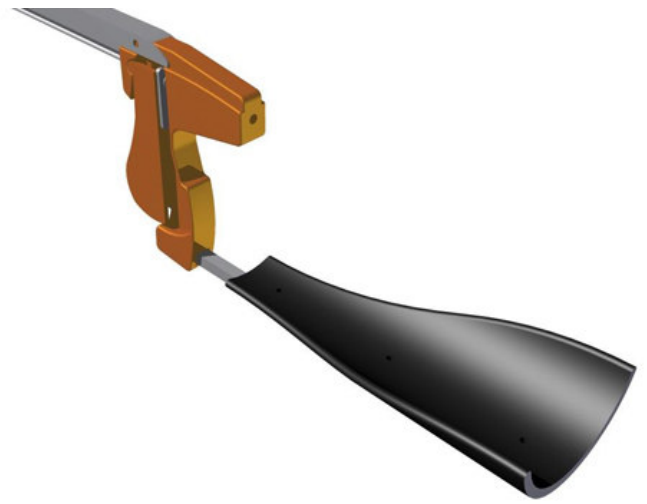
Figure 1.a. 3D model of a supporting part for a “helping hand”.
