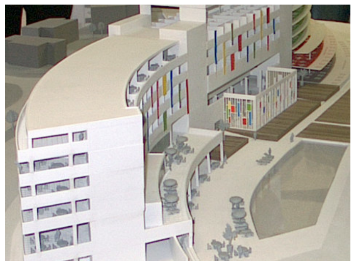
Figure 4.b. Prototype of the kemer building using RP
